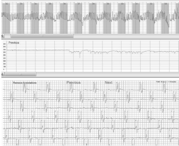
Figure 1. A sample multi-scale plot. The top panel shows long-term heart rate with light and dark cycles. Each data point represents 10 minutes of averaged heart rate. In the middle panel is the instantaneous heart rate comprising the 10-minute averaged data point most recently clicked in the top plot. The bottom plot shows the first segment of ECG corresponding to the time of interest. The user may browse the ECG chart with the previous and next buttons.
